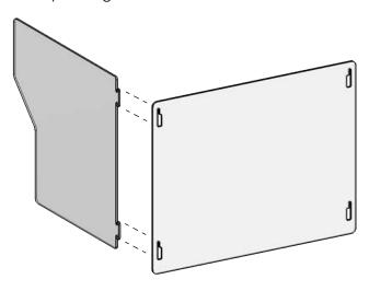
**STEP 3:** Insert hooks of Side Panel into the largest opening in slots on Front Panel.
